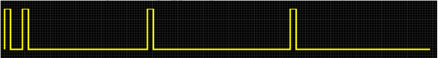
Daihatsu +1 cam wheel arrangement. Fill in. Patterns 3 + 1 and 4 + 1 used in Daihatsu 3 and 4 cylinder
